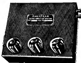
*Complete 2 stage audio amplifier with first stage AmerTran De Luxe for UX 227 AC and second stage AmerTran Push-Pull for two 171 or 210 power tubes. Operates with 450 volt AmerTran Hi-Power Box. Price east of Rockies—less tubes—$80.00.
